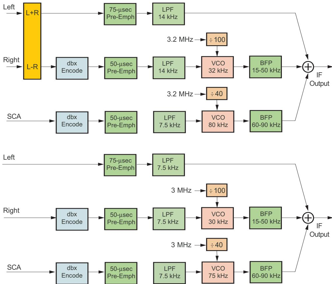
Figure 3 – Signal processing chain for each channel of the FM modulator: stereo and non-stereo options
