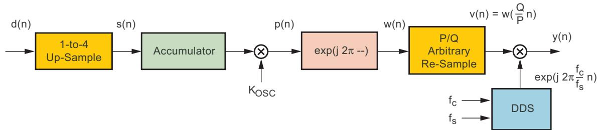
Figure 4 – Signal flow diagram: DSP-based complex baseband FM modulator
