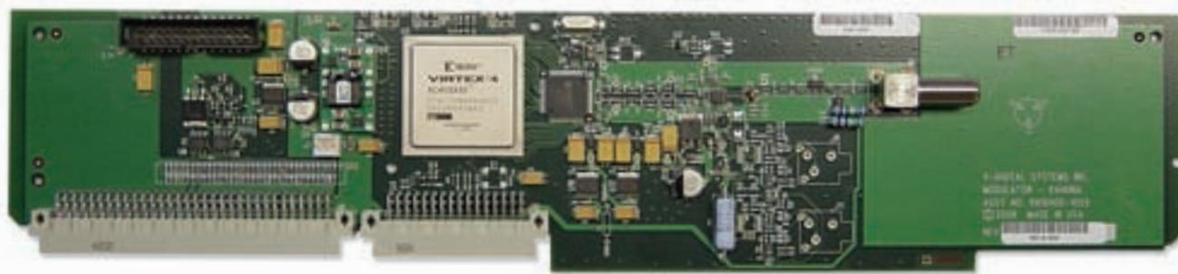
*Figure 7 – Re-modulator board showing Xilinx Virtex-4 FPGA that implements 384 FM modulators implemented on 192 modulator boards in the equipment bay shown in Figure 1.*
